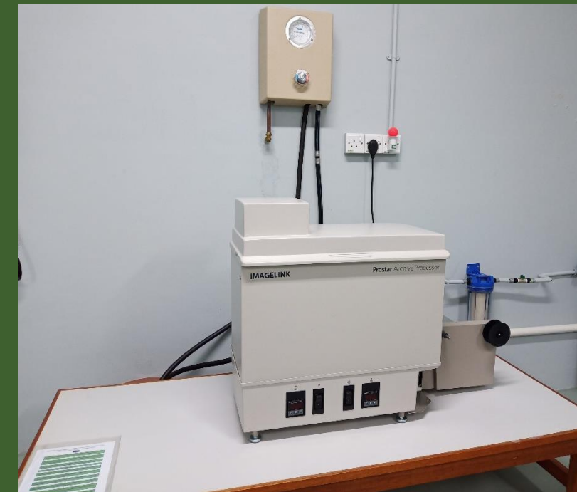
Imagelink Film Processor - for developing microfilm.
