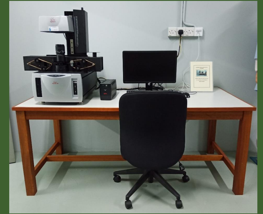
Sunrise Apollo Microfilm Scanner - for scanning of microfilm to digital images.
