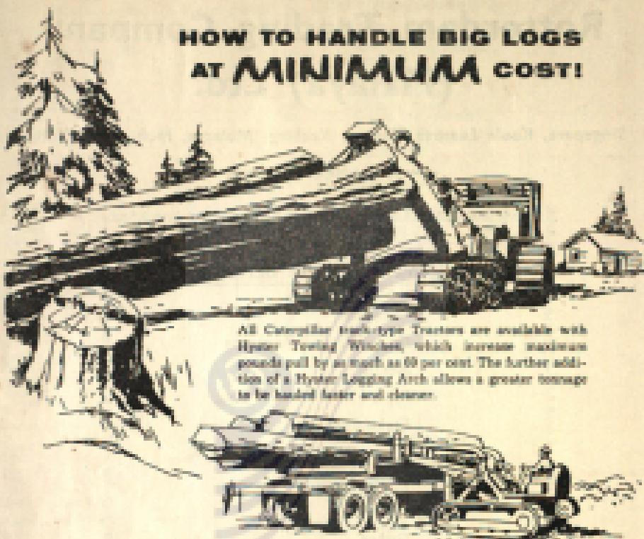
All Caterpillar track-type Tractors are available with Hydram Towing Winches, which increase maximum pounds pull by as much as 60 per cent. The further addition of a Hydrom Logging Arch allows a greater tonnage to be hauled faster and clearer.
