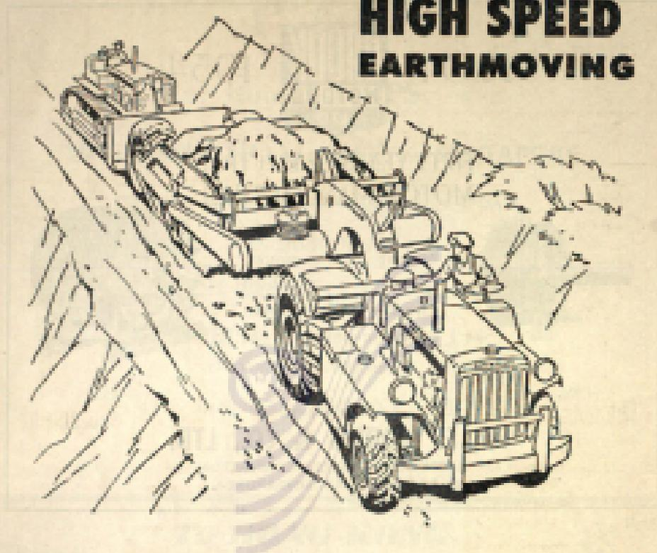
A Caterpillar DW10 Tractor with a No. 10 Scraper provides dependable, high speed hauling. These matched units have an available top speed of 24.5 MPH. The No. 10 Scraper has a capacity of 8.7 cu. yds. struck and 11 cu. yds. heaped. With this tractor-scraper, cycle time is cut to a minimum. The No. 10 Scraper provides positive ejection of the stickiest materials.
