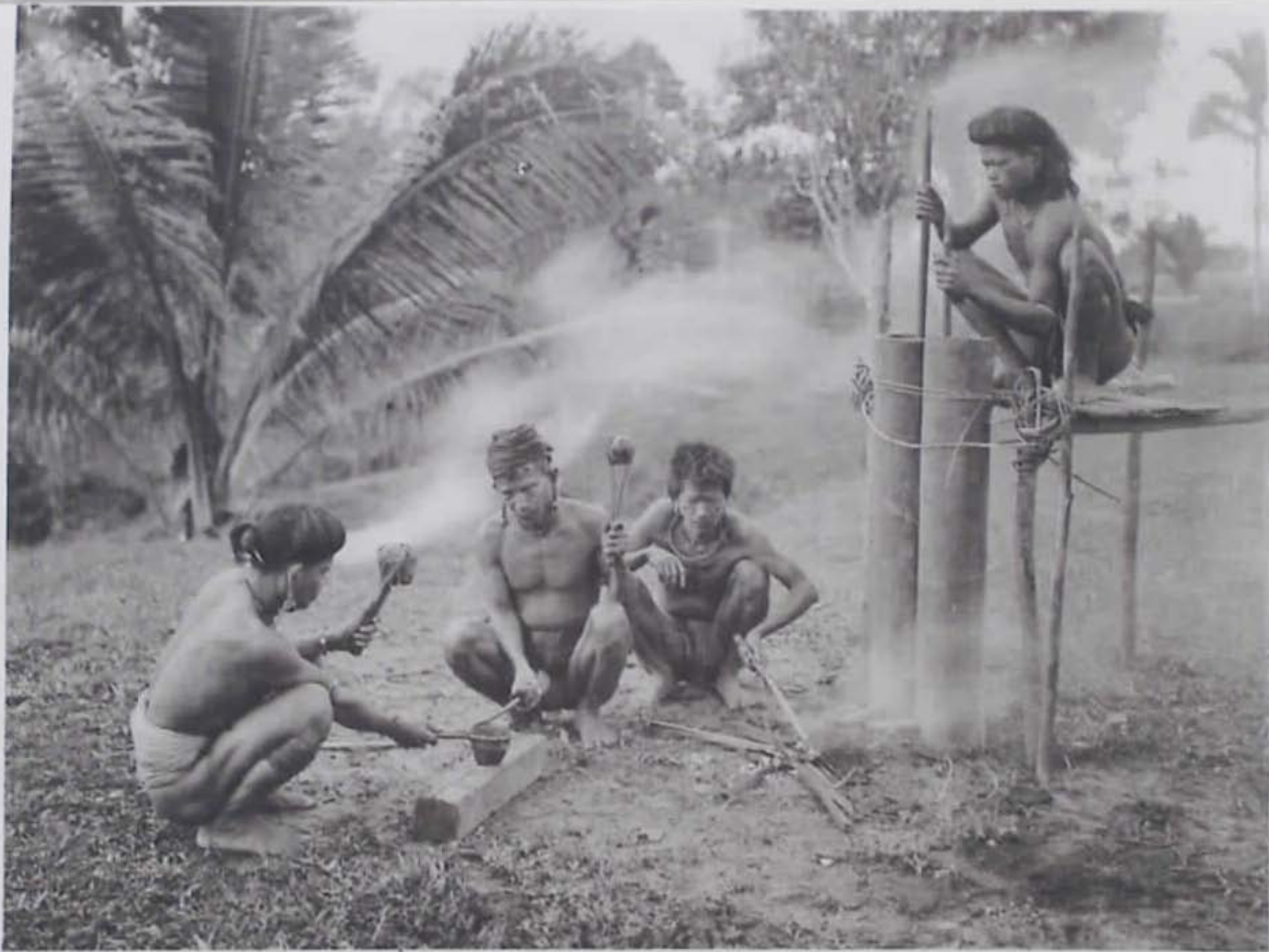
PLATE 107. KALABIT SMITHS USING STONE HAMMERS.
